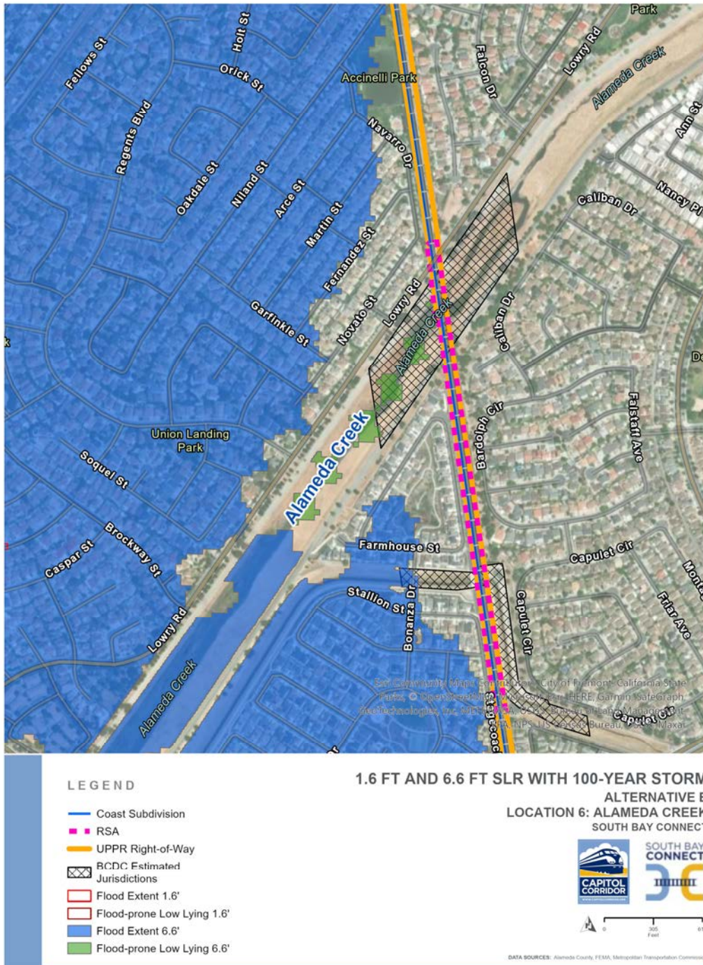
Figure 20. 1.6-Foot and 6.6-Foot Sea Level Rise Inundation with Baseline MHW and 100-Year Storm Event at Location 6
